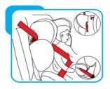
Step 3: Pull the vehicle safety belt and pass through the belt path, and then buckle it up. Position shoulder belt through the shoulder belt guide as shown in photo.
