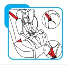
Step4.Place your knee on the base of the safety seat and grip the top piece of seat belt webbing.Pull the webbing upwards to tighten the seat belt. then you can place your child into the safety seat. Check the height of the shoulder straps on the correct position.
