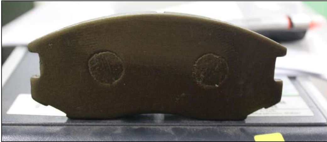
Figure 11 Brake pad CF9 without back plate marking
