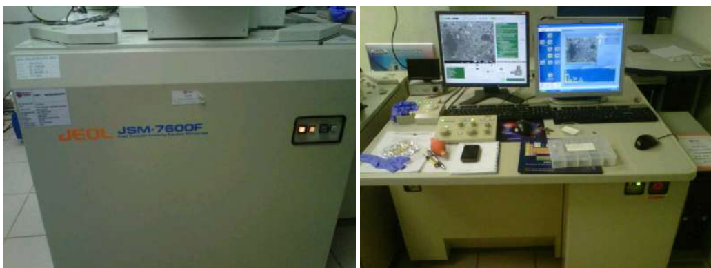
Figure 4 JEOL JSM 7600F FESEM attached with EDX
