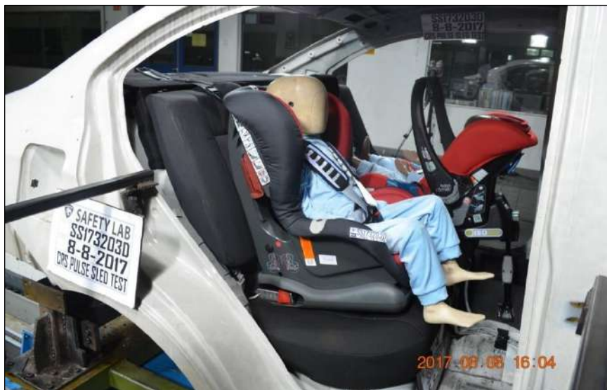
Figure 2 Sled test set up for CRS and dummies
